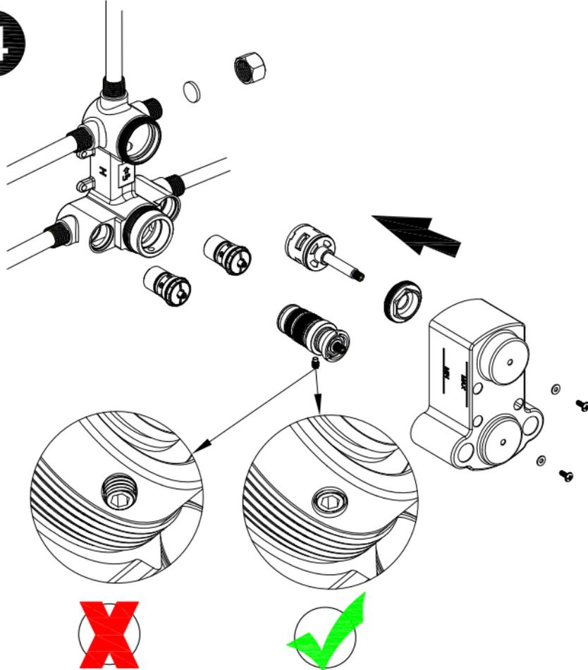
Reinstall the valve components into their original positions.
