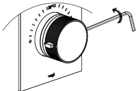
With the handle still turned to its maximum, tighten the set screw with the help of an allen key, securing the handle.
