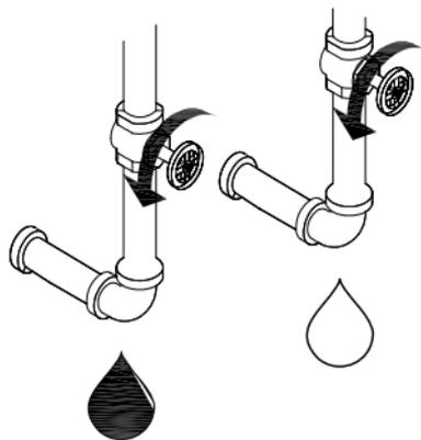
After welding, purge the water supply system for around 30 seconds.
