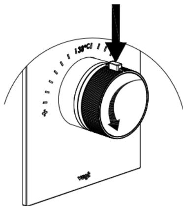
Press the security button and turn the handle counterclockwise until stopped.
