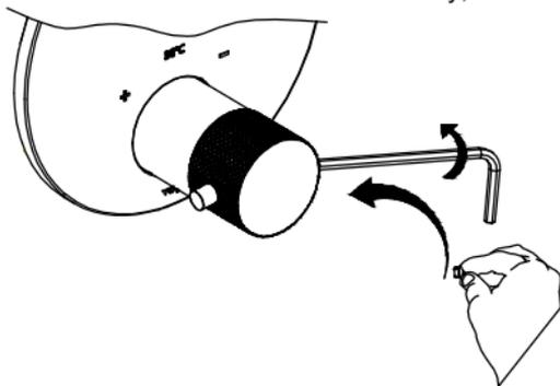
With the handle still turned to its maximum, tighten the set screw with the help of an allen key, securing the handle.
