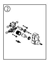
If welding is involved you must remove internal valve components prior to the welding. Please note the original position of the cartridge.
