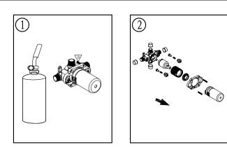
If welding is involved you must remove internal valve components prior to the welding. Please note the original position of the cartridge.
