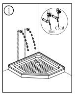
Purge the water supply system for around 30 seconds.
