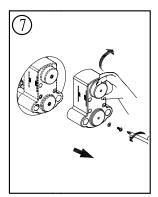
Remove the screws and take the plastic cover off the valve.
