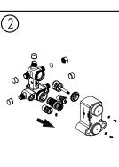
If welding is involved you must remove internal valve components prior to the welding. Please note the original position of the cartridge.
