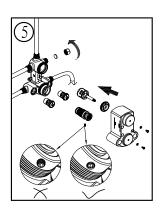
Reinstall the valve components into their original positions.
