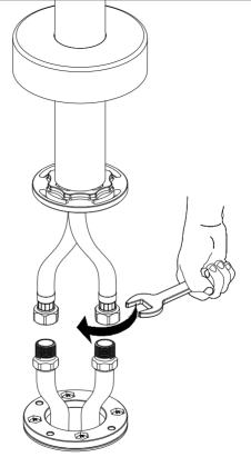
Connect the cold and hot water inlets, and check watertightness.
