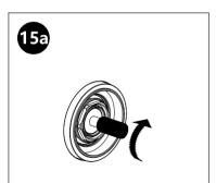
Contrarotate - Closed By turning the cartridge (greyed part)
