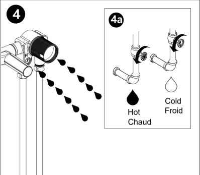
Purge the water supply system for around 30 seconds.
