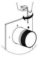
Tighten the set screw with the help of an allen key, securing the handle.
