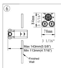
Make sure that the valve is installed in such a way that the finished wall is between the Max and Min marks.
