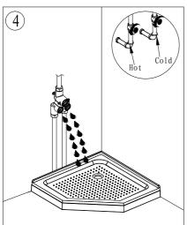
Purge the water supply system for around 30 seconds.
