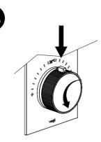
Press the security button and turn the handle counterclockwise until stopped.
