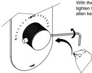
With the handle still turned to its maximum, tighten the set screw with the help of an allen key, securing the handle.
