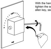
With the handle still turned to its maximum, tighten the set screw with the help of an allen key, securing the handle.
