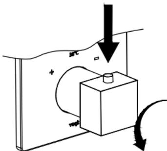
Press the security button and turn the handle counterclockwise until stopped.
