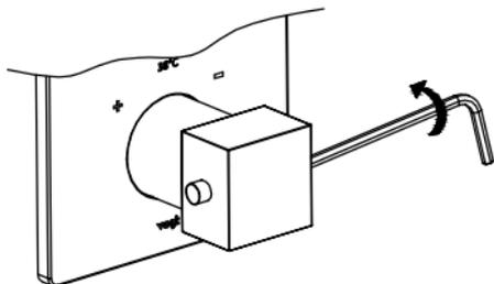
With the handle still turned to its maximum, tighten the set screw with the help of an allen key, securing the handle.
