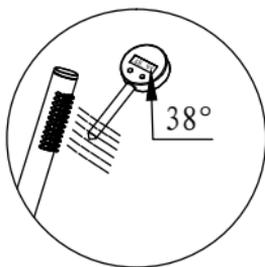
With a thermometer, calibrate the water exiting the hand shower to 38° (max) by turning the cartridge (greyed part).
