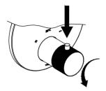
Press the security button and turn the handle counterclockwise until stopped.
