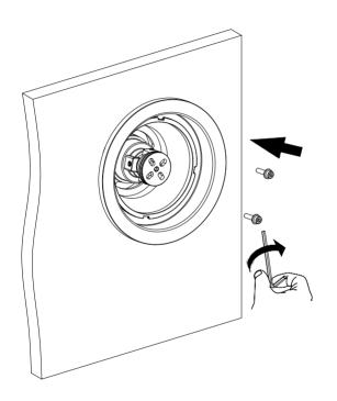
Lock the main body on the connector with the M4x20 Screws.
