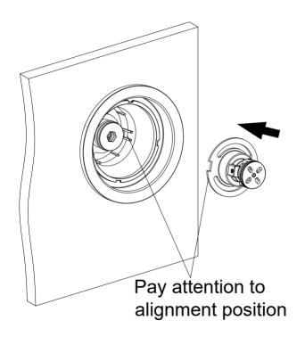
Install the main body as shown in the diagram
