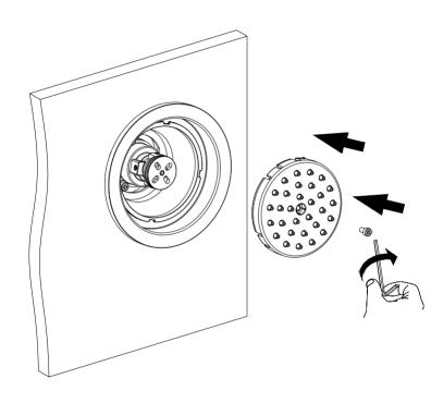
Lock the nozzle plate on the main body with the M4x12 Screws.
