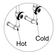
Purge the water supply system for around 30 seconds.
