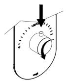
Press the security button and turn the handle counterclockwise until stopped.
