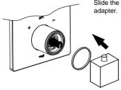
Slide the temperature handle onto the cartridge adapter.
