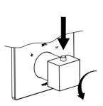
Press the security button and turn the handle counterclockwise until stopped.
