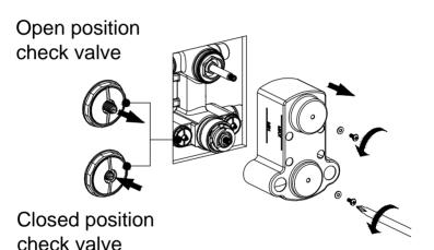
Do not over tighten when closing or opening
