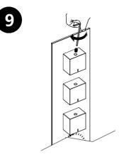
Tighten the set screw with the help of an allen key, securing the handle.
