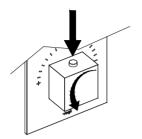
Press the security button and turn the handle counterclockwise until stopped.
