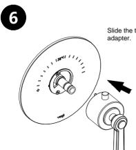
Slide the temperature handle onto the cartridge adapter.
