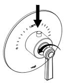
Press the security button and turn the handle counterclockwise until stopped.
