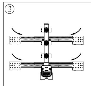
Once you have your valve, adjust the valve to the center of the bracket, by sliding the square nuts through the slot opening of your brackets.
