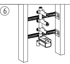
FOR 2X4 INSTALLATION \*\*\*\*It is imperative that the brackets are installed all the way to the back of the 2X4 frame to ensure a proper installation.\*\*\*\*
