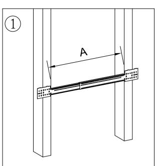
Measure the distance(A) between your studs.Grab provided brackets adjust accordingly to the distance measured.
