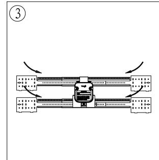
Once you have your valve, adjust the valve to the center of the bracket, by sliding the square nuts through the slot opening of your brackets.
