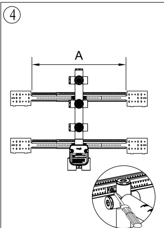
4 Once you have remeasured the length of brackets to the length of the stud frame. Fasten the valve body to the brackets.
