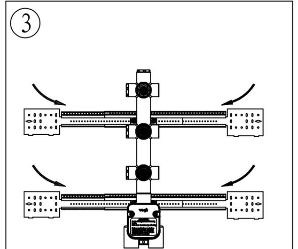
3 Once you have your valve, adjust the valve to the center of the bracket, by sliding the square nuts through the slot opening of your brackets.
