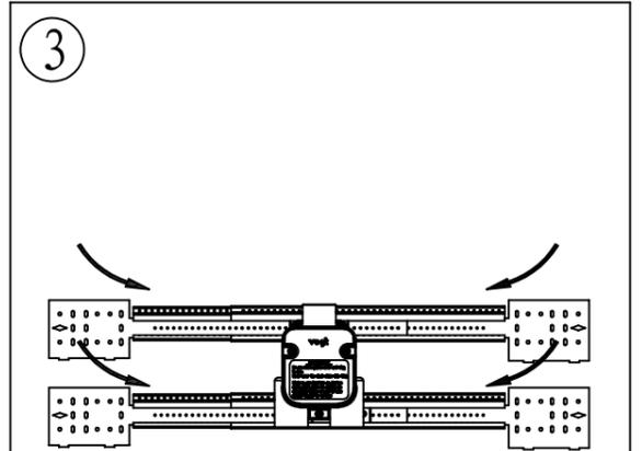
③ Once you have your valve, adjust the valve to the center of the bracket, by sliding the square nuts through the slot opening of your brackets.
