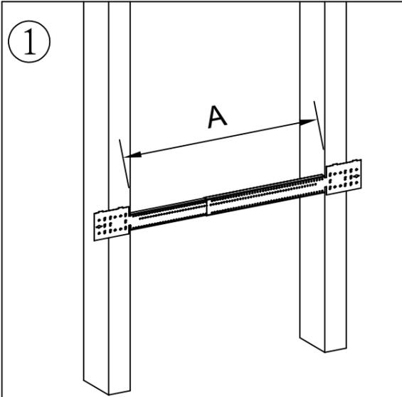
1 Measure the distance(A) between your studs. Grab provided brackets adjust accordingly to the distance measured.
