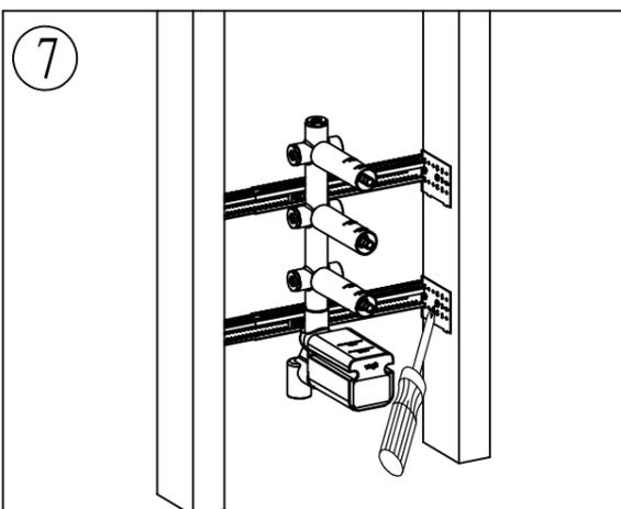
7 Secure the brackets to the frame on either side.
