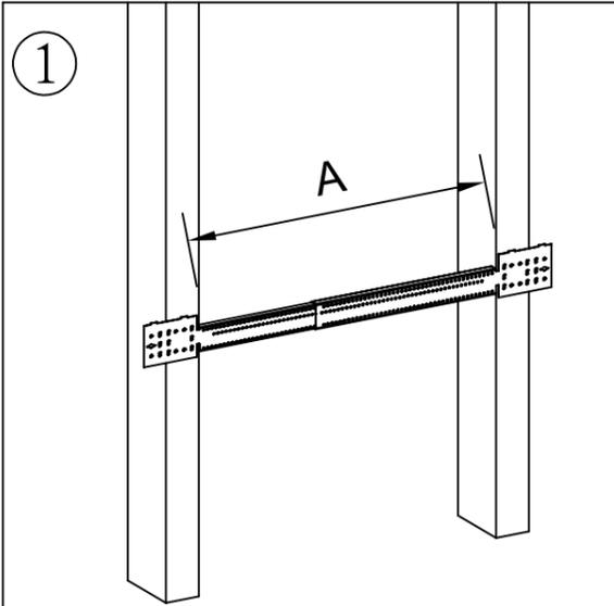
① Measure the distance(A) between your studs. Grab provided brackets adjust accordingly to the distance measured.
