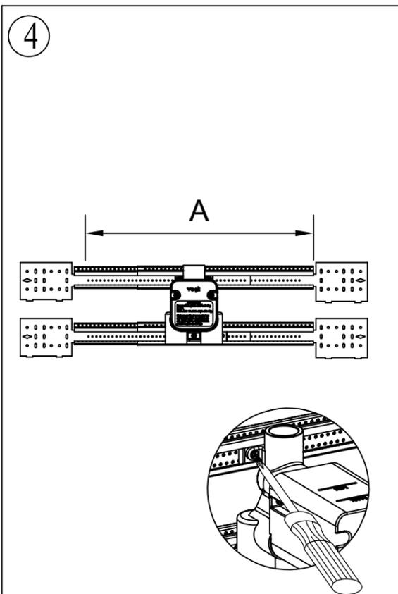
④ Once you have remeasured the length of brackets to the length of the stud frame. Fasten the valve body to the brackets.
