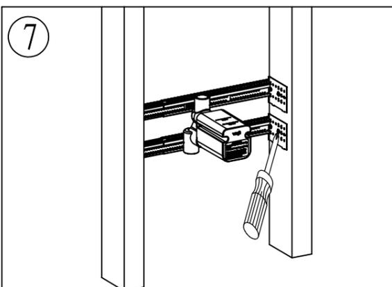
⑦ Secure the brackets to the frame on either side.
