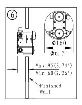
Make sure that the valve is installed in such a way that the finished wall is between the Max and Min marks.
