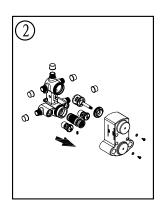
If welding is involved you must remove internal valve components prior to the welding. Please note the original position of the cartridge.
