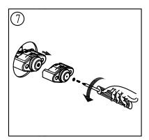
Remove the screws and take the plastic cover off the valve.
