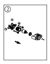
If welding is involved you, must remove internal valve components prior the welding. Please note the original position of the cartridge.
