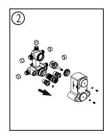
If welding is involved you must remove internal valve components prior to the welding. Please note the original position of the cartridge.
