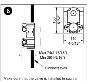
Make sure that the valve is installed in such a way that the finished wall is between the Max and Min marks.
