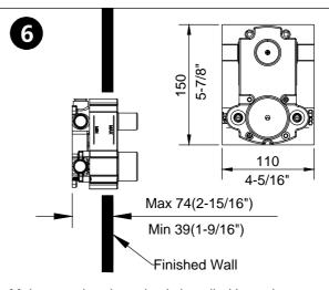
Make sure that the valve is installed in such a way that the finished wall is between the Max and Min marks.
