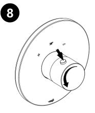
Press the security button and turn the handle counterclockwise until stopped.
