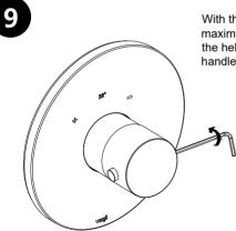
With the handle still turned to its maximum, tighten the set screw with the help of an allen key, securing the handle.
