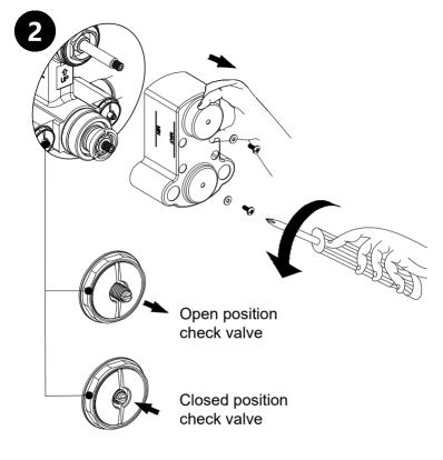
Do not over tighten when closing or opening
