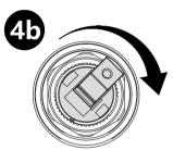
While measuring the water temperature, turn the control clockwise until you reach 49°C.
