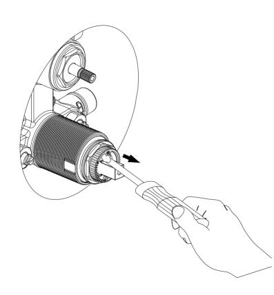
Use a tool to remove the limiting temperature device.
