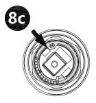
Replace the limiting temperature device so that it prevents the cartridge from turning further.
