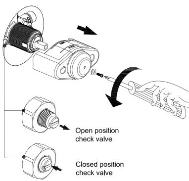
Do not over tighten when closing or opening
