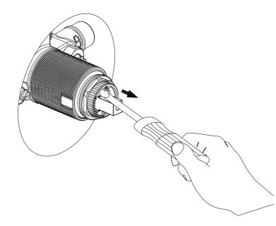
Use a tool to remove the limiting temperature device.
