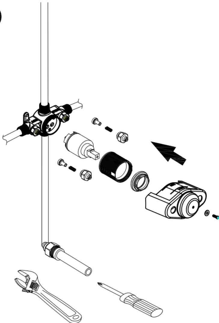
Reinstall the valve components into their original positions.
