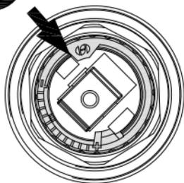
Replace the limiting temperature device so that it prevents the cartridge from turning further.
