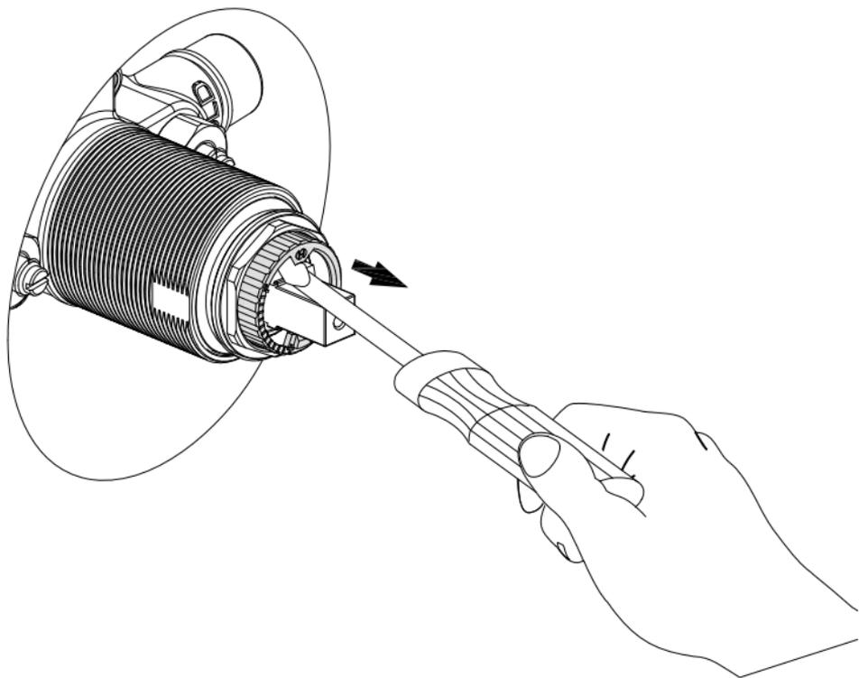
Use a tool to remove the limiting temperature device.
