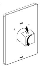
Press the security button and turn the handle counterclockwise until stopped.
