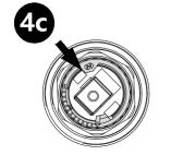
Replace the limiting temperature device so that it prevents the cartridge from turning further.
