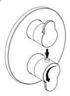
Press the security button and turn the handle counterclockwise until stopped.
