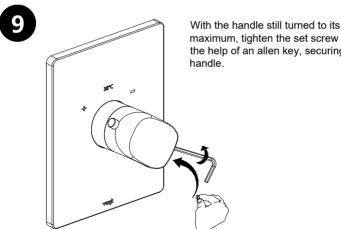
maximum, tighten the set screw with the help of an allen key, securing the
