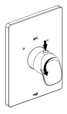
Press the security button and turn the handle counterclockwise until stopped.
