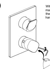
With the handle still turned to its maximum, tighten the set screw with the help of an allen key, securing the handle.
