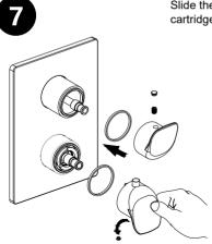
Slide the temperature handle onto the cartridge adapter.
