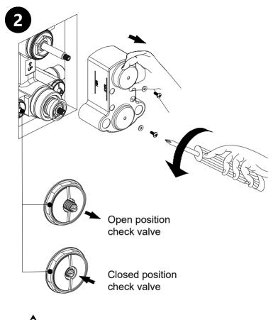
Do not over tighten when closing or opening
