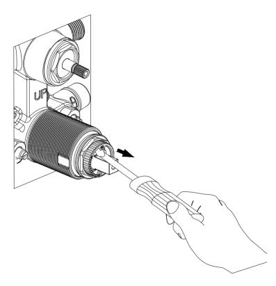
Use a tool to remove the limiting temperature device.
