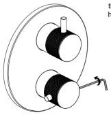
With the handle still turned to its maximum, tighten the set screw with the help of an allen key, securing the handle.
