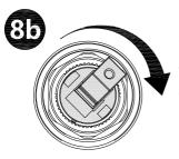
While measuring the water temperature, turn the control clockwise until you reach 49°C.
