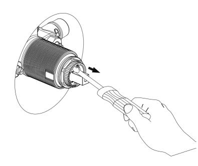
Use a tool to remove the limiting temperature device.
