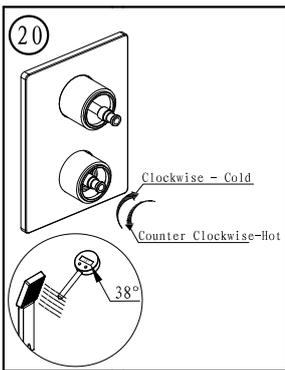
Use a thermometer to calibrate the cartridge. Make sure the water temperature is at 38° C.
