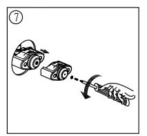
Remove the screws and take the plastic cover off the valve.
