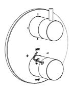
With the handle still turned to its maximum, tighten the set screw with the help of an allen key, securing the handle.
