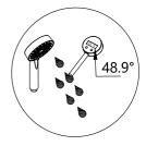
With a thermometer, calibrate the water exiting the handle shower to 48.9° (max) by turning the cartridge (greyed part).
