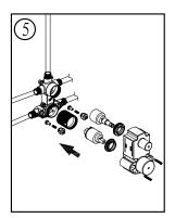
Reinstall the valve components into their original positions.
