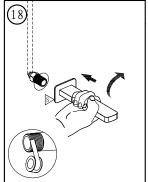
Use a thermometer to calibrate the cartridge. Make sure the water temperature is at 38° C.
