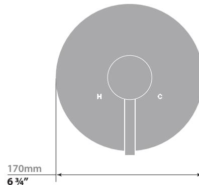
**VE.110 - Pressure Balanced Valve Without Diverter**
