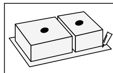
6. Lower the sink into the cutout hole. Fix the sink by tightening mounting clips with the screwdriver.
