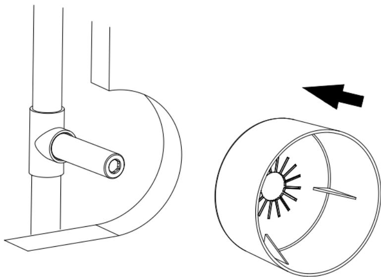
Install the plastic cover as shown in the diagram
