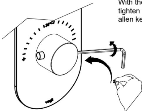
With the handle still turned to its maximum, tighten the set screw with the help of an allen key, securing the handle.
