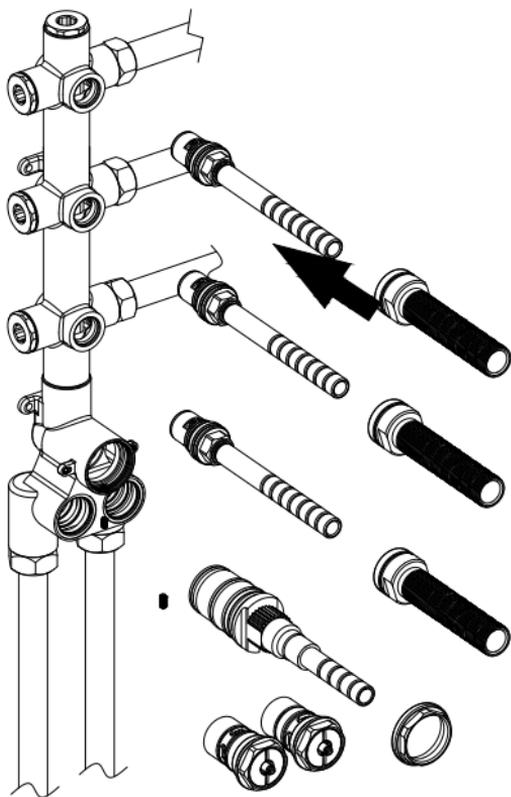
Reinstall the valve components into their original positions.
