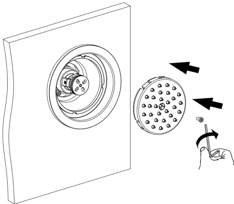
Lock the nozzle plate on the main body with the M4x12 Screws.
