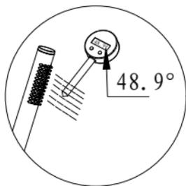
With a thermometer, calibrate the water exiting the hand shower to 48.9° (max) by turning the cartridge (greyed part).
