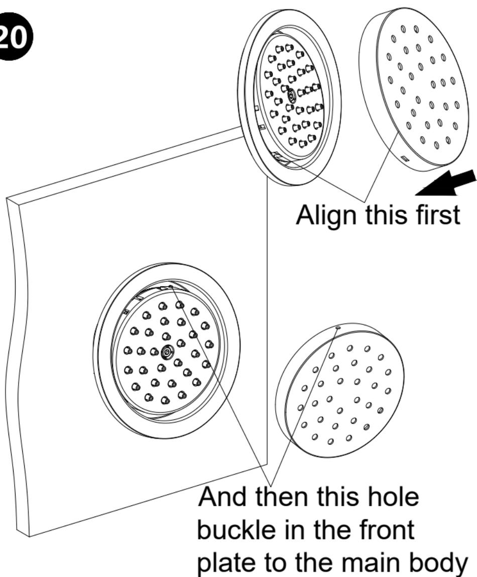
Install the front plate as shown in the diagram
