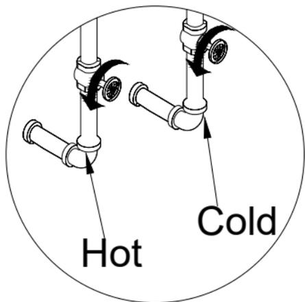
Purge the water supply system for around 30 seconds.
