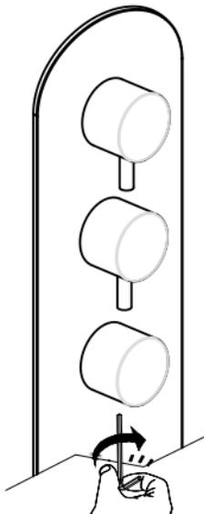
Tighten the set screw with the help of an allen key, securing the handle.
