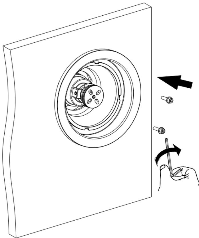
Lock the main body on the connector with the M4x20 Screws.
